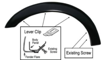
Place the flare on the vehicle. Apply 3 Lever Clips, secure it to the hole with existing screws as shown. Fasten the existing factory 2 screws into the original location that were previously removed.
