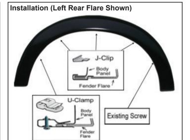
Place the flare on the vehicle. Apply 3 J-Clips into the mounting slots in the flare and secure it to the vehicle, 1 U-Clamp secures into the hole with flat head screws as shown. Fasten the existing 3 factory screws into the original location that were previously removed.
