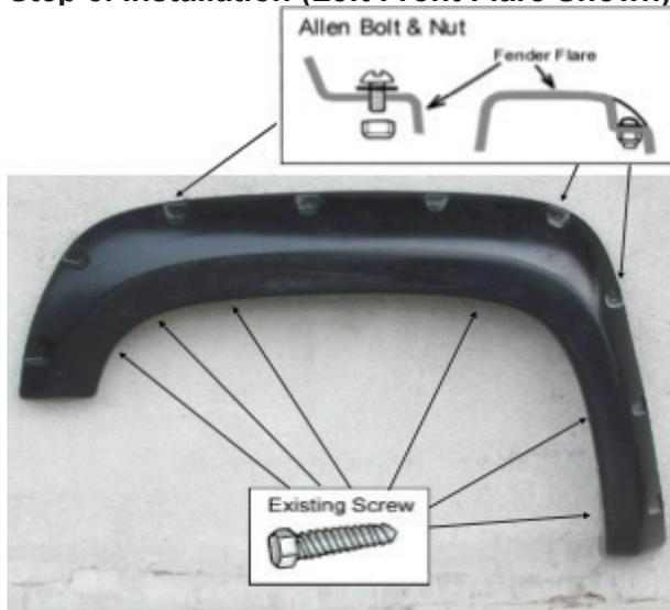
Use torx bit to tighten allen bolt & put firmly on every pocket of the fender flares. **DO NOT OVER TIGHTEN!** Remove 6 existing screws from the fasteners on the vehicle. Place the flare on the vehicle. Reinstall the existing factory screws into the original location that were previously removed. Do not tighten the screws fully until the flare are aligned and extrusive against the body.
