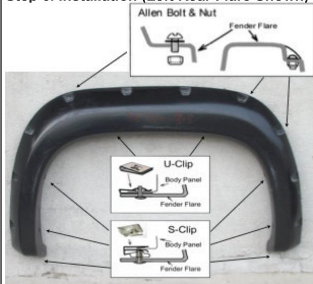
Use torx bit to tighten allen bolt & put firmly on every pocket of the fender flares. **DO NOT OVER TIGHTEN!** Hold the flare in position on the vehicle, use a grease pencil to mark eight hole locations. Apply 2 U-Clips over two top marks, align with holes in flare. Apply 6 S-Clips over six lower marks, align with holes in flare. Adjust the clips in position, use 2 flange screws and 6 truss machining screws to secure it as shown.
