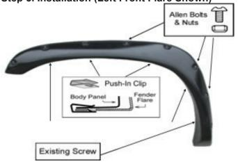
Use torx bit to tighten allen bolt & put firmly on every pocket of the fender flares first. Place the flare on the vehicle. Apply 2 Push-In Clips into the mounting slots in the flare and secure it to the vehicle as shown. Fasten the existing factory screws into the original location that were previously removed.
