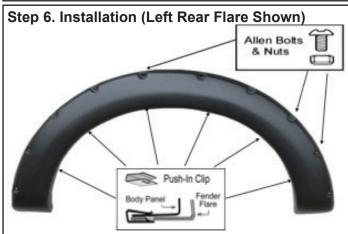
Use torx bit to tighten allen bolt & put firmly on every pocket of the fender flares. Place the flare on the vehicle. Apply 6 Push-In Clips into the mounting slots in the flare and secure it to the vehicle as shown.
