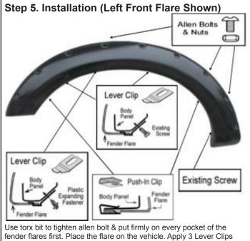
fender flares first. Place the flare on the vehicle. Apply 3 Lever Clips secure it to the hole with 2 existing screws and 1 expanding fastener. Apply 2 Push-In Clips into the mounting slot in the flare and secure it to the vehicle. Fasten the existing factory screw into the original location that were previously removed.
