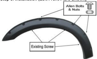
Use torx bit to tighten allen bolt & put firmly on every pocket of the fender flares. Place the flare on the vehicle. Fasten the existing factory screws into the original location that were previously removed.
