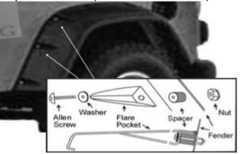
Use right tool to remove rear wheel well skirting and factory fender flares. Place all allen screws, washers through pocket hole, place the spacer on the screw from back side of the pocket as shown. Place the flare on the vehicle with best position and flush against the vehicle. Insert the allen screws through the factory holes on the fender, use hex key to tighten allen screw & put firmly on every pocket of the fender flare. Do not tighten it until all crews have been installed.
