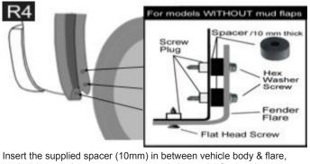
apply 2 hex washer screws on top two holes and 1 flat head screw on bottom hole, and secure the flare to the body.
