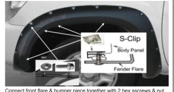
Connect front flare & bumper piece together with 2 hex sscrews & nut (left illustration). Hold the flare firmly and mark 4 clips locations through the existing holes on the flare and remove the flare. Apply 4 S-Clips over 4 marks and place the flare on the vehicle. Secure 4 machine screws into the S-Clip.
