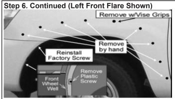
Remove 8 factory clips by hand on the fender. Remove 1 factory clip with vise grips on the fender as shown. Remove factory plastic screws on the front of wheel well, use screwdriver and pry it out (bottom illustration).
