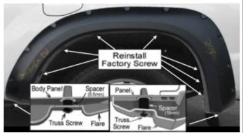
Reinstall 7 factory screws. Install supplied truss screws (20mm) through spacer (6.5mm) into factory hole on the bottom of the front end, as left shown. Install supplied truss screws (50mm) through spacer (19mm) into factory hole on the bottom of rear end, as right shown.
