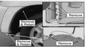
Remove 2 existing screws from the factory flare/bumper piece/small part) as top left shown, save screws for reinstallation. Remove 2 factory screws from the underneath of the factory bumper cover, pull down the bumper cover and splash shield (bottom left illustration), save screws for reinstallation. Remove 5 factory plastic clips from the inside of the factory bumper cover (bottom illustration). Pull away the factory flare (bumper piece/small part) from the vehicle.
