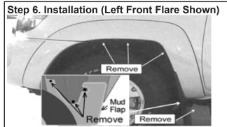
Remove 3 existing screws from the mud flap, save screws for reinstallation (see illustration). Remove 3 factory screws on the top of the flare lip & 1 screw from the bottom as shown, save screws for reinstallation. Pull away the factory flare (large part) from the vehicle.
