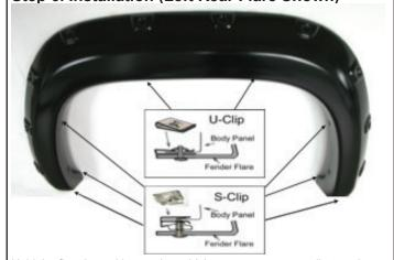
Hold the flare in position on the vehicle, use a grease pencil to mark eight hole locations. Apply 2 U-Clips over two top marks, align with holes in flare. Apply 6 S-Clip over six lower marks, align with holes in flare. Adjust the clips in position, use 2 flange screws and 6 truss machine screws to secure it as shown.
